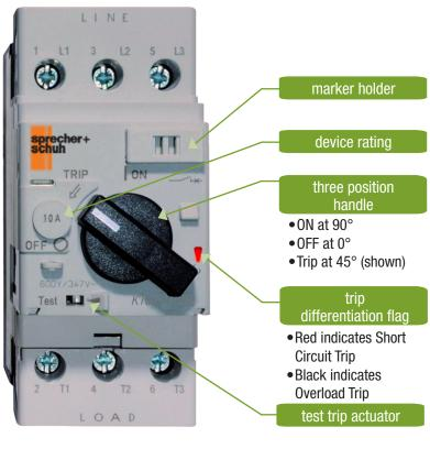
Sprecher + Schuh's new KTU7 series of UL Molded Case Circuit Breakers provide reliable thermal and magnetic over current protection. This series is UL489 Listed, CSA22.2 No. 5 and IEC 60947-2 compliant for global applications. The current limiting circuit breaker provides fixed short circuit and overcurrent protection and offers high interrupting ratings for 2- and 3-pole devices from 0.5 to 30A. These Circuit breakers are 100% rated up to 10A.
