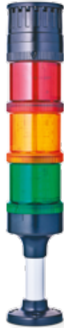
Order number: ECO70-Q81 Colours: red/orange/green Function: LED steady beacon, buzzer steady or pulsing tone Nominal voltage: 230 V AC Type of mounting: Tube mounting (100 mm tube length)
