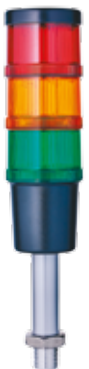
Order number: C70-Q601 Colours: red/orange/green Function: LED steady beacon Nominal voltage: 24 V AC/DC Type of mounting: horizontal Length: 100 mm
